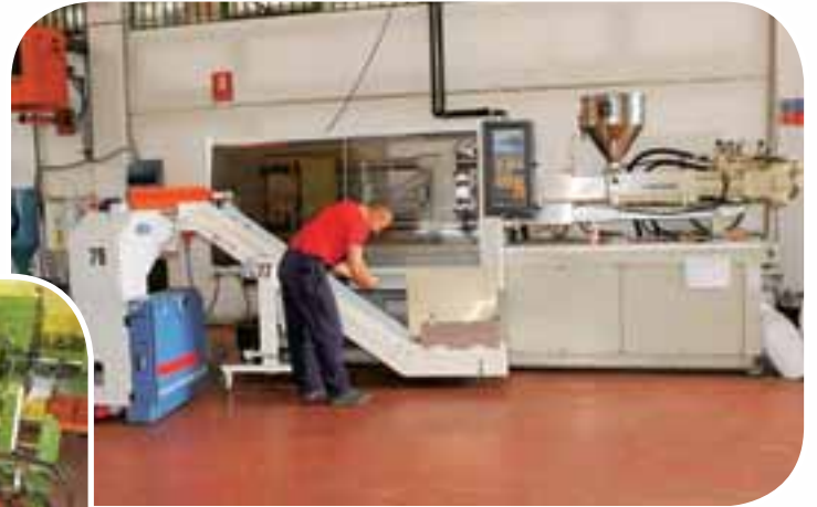
Stampaggio materie plastiche Presswork of Plastic Materials
